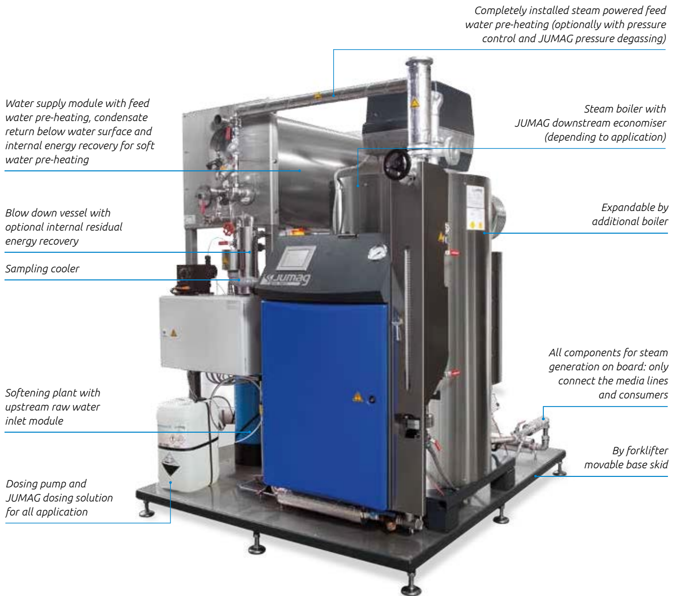
Fig.: Compact steam boiler, example configuration
